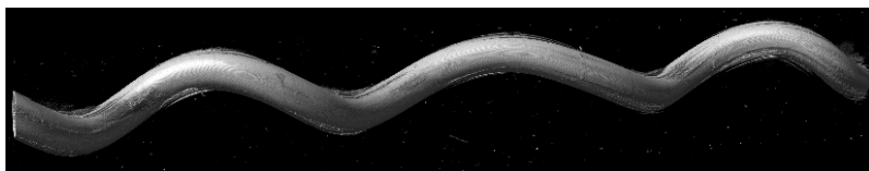
(a) Wound silver wire current collector inside a CNT-microtube.
