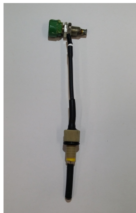
(b) Photo of the self-made reference electrode
