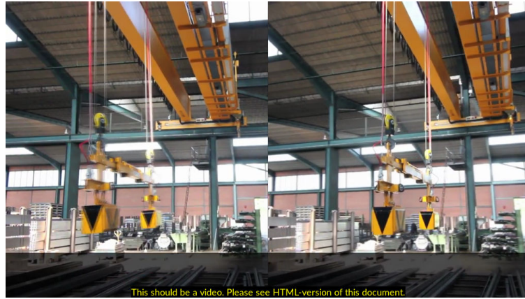
Figure 5.4: Sway control in a gantry crane by SWF [70].
