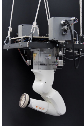
Figure 6.21: Hardware SPCM prototype with attached robot. Gyros are in the aluminum cases with the gyro motors mounted on their sides. The gimbal motors hang underneath the gyros. The motor controller and power supply are mounted underneath the platform. The gyro controller, IMU and communication interface for these are mounted on top. Note that the rope suspension was rotated by 90^\circ for the picture.
