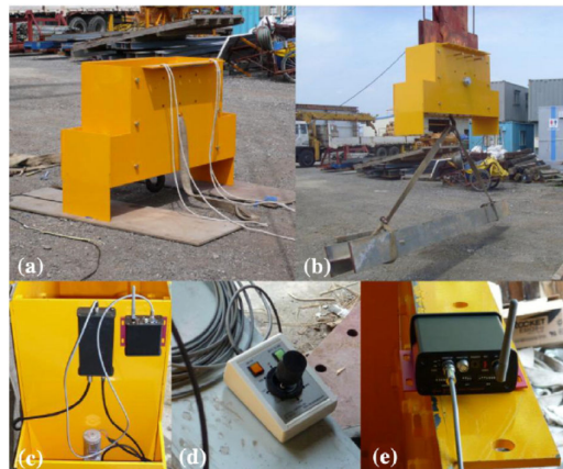
Figure 2.14: Motorized crane hook experiments [64].
