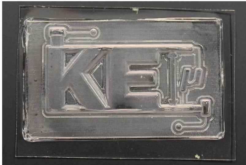
Figure 4.4: Thermoformed foil with structures for cavities and micro channels.
