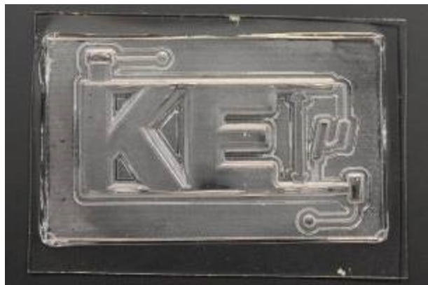
Figure 3.38: A good sample fabricated by ultrasonic thermoforming.
