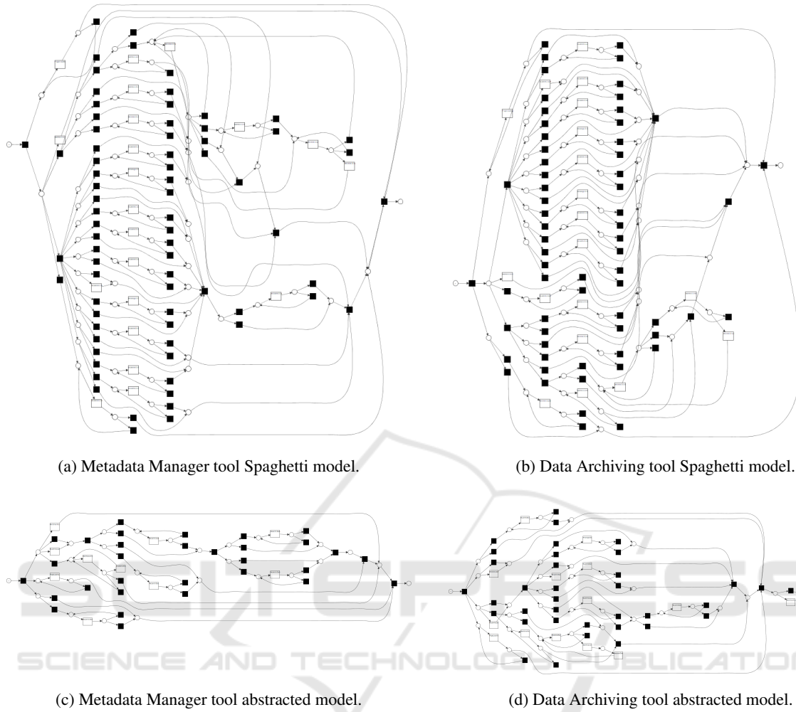
Figure 2: The discovered Petri net models before and after applying the event log abstraction technique.
