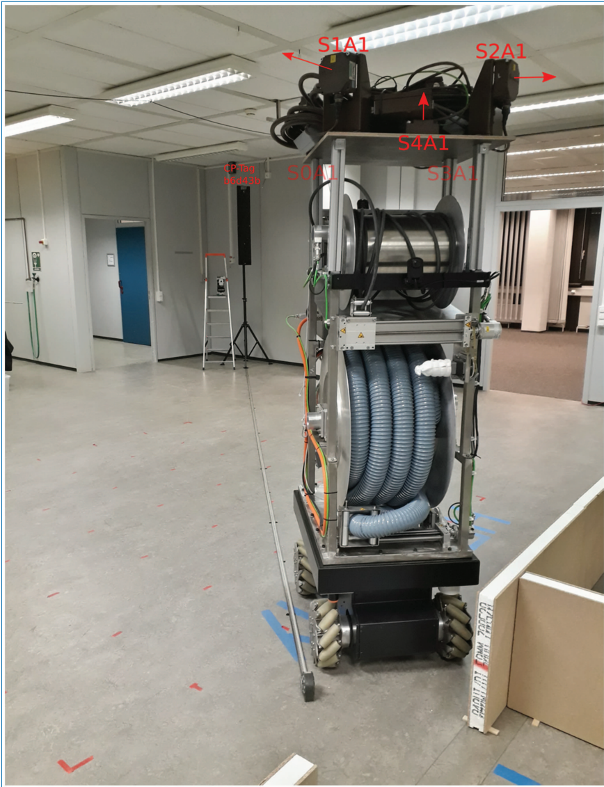
Figure 3.115. Mounting positions and orientation of iRTT-AUs and CP-Tag.
