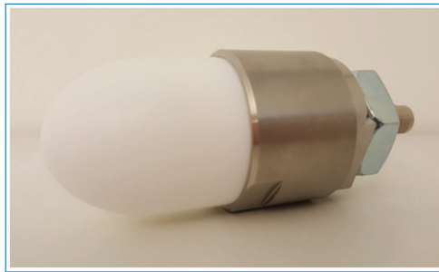
Figure 3.163. iLDR-C front view showing the PTFE lens.
