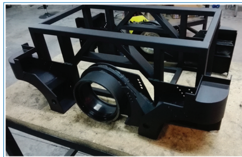
Figure 3.55. Frame after being blued and painted.
