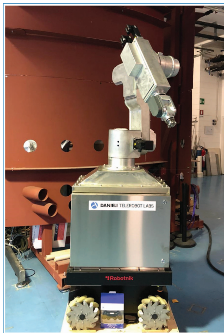
Figure 3.181. Robot arm integrated on the robotic platform.
