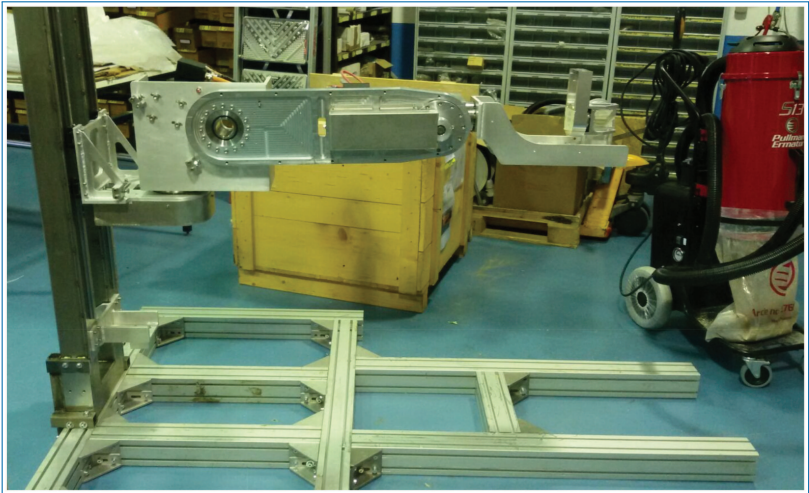
Figure 3.82. Complete arm structure on dummy frame structure ready for electrical integration.
