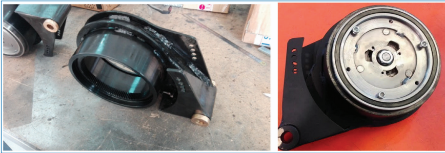
Figure 3.61. Hub and Rocker arm finished with Bronze bearing inserted.
