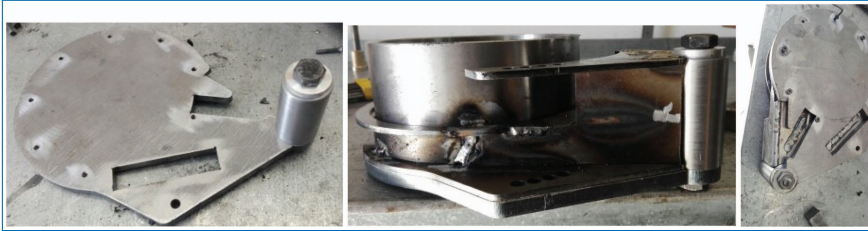
Figure 3.60. Plinth used for soldering rocker arm to Lathe machined motorwheel hub.
