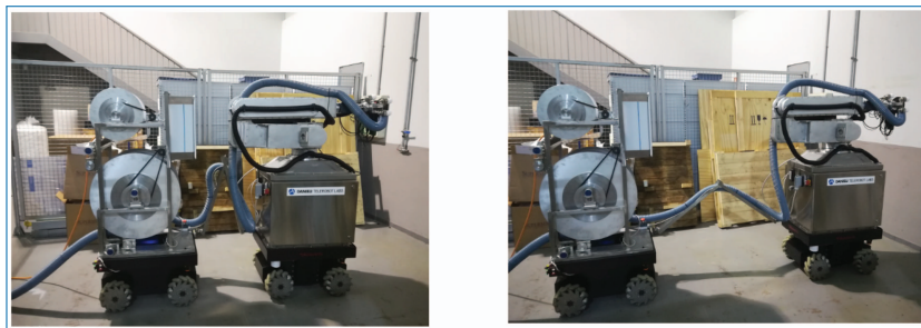
Figure 4.16. Robotic Tandem with cable and aspiration bridge.
