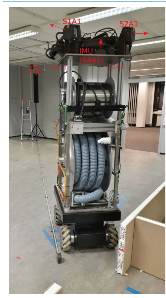
Figure 4.44. Mounting positions and orientation of iRTT-AUs and CP-Tag.
