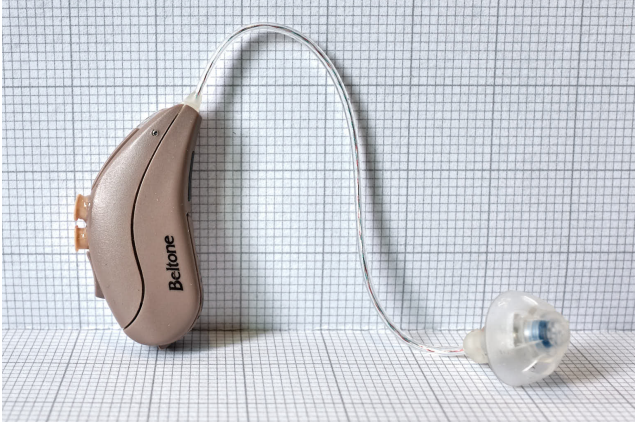
(b) Photo showing the plugs for the connection cables (left side), with open dome attached to the HA receiver. (Taken from [17], licensed under CC BY 4.0, and adapted.)
