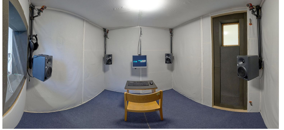
Figure 10: Custom-made hearing booth. (Photo taken from [17], licensed under CC BY 4.0, and adapted.)
