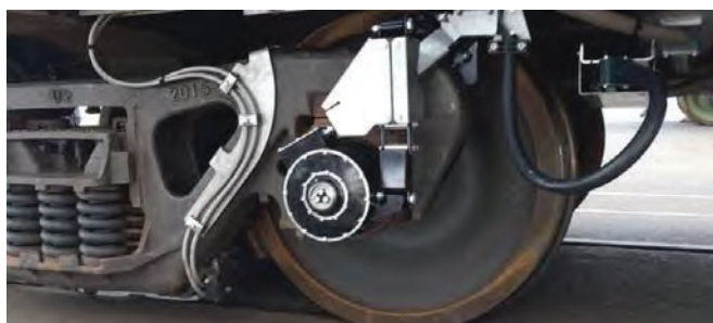
Figure 3: Axle end generator for power supply
