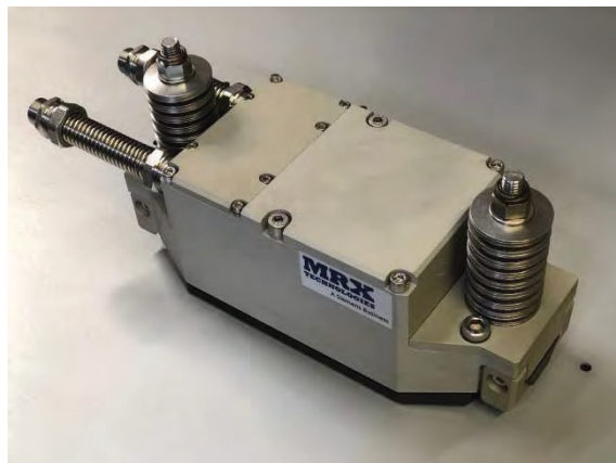
Figure 1: Siemens Mobility Broken Rail Detection (BRD) sensor
