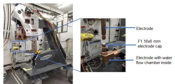
Figure 1: Fronius 'C-type' resistance spot welding machine along with F1 16*6 mm electrode caps
