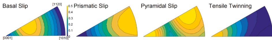
Figure 8. Theoretical calculated Schmid Factors as a function of grain orientation for uniaxial tension, displayed as inverse polfigures.
