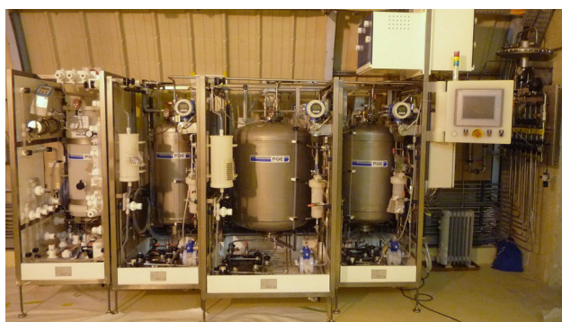
Fig. 9 Detector Fluid Operating System installed in the underground laboratory of the far detector. From left to right are shown: Target, GC, buffer and veto liquid systems; the control unit including touch screen; the over-, underpressure safety and low pressure nitrogen boxes, and one of the gas system manifolds
