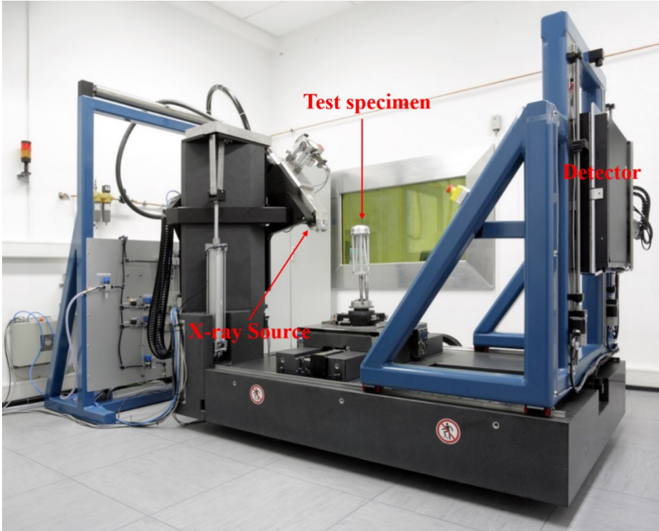
Fig. 3-7. Open X-ray computed tomography system at ZEA-1
