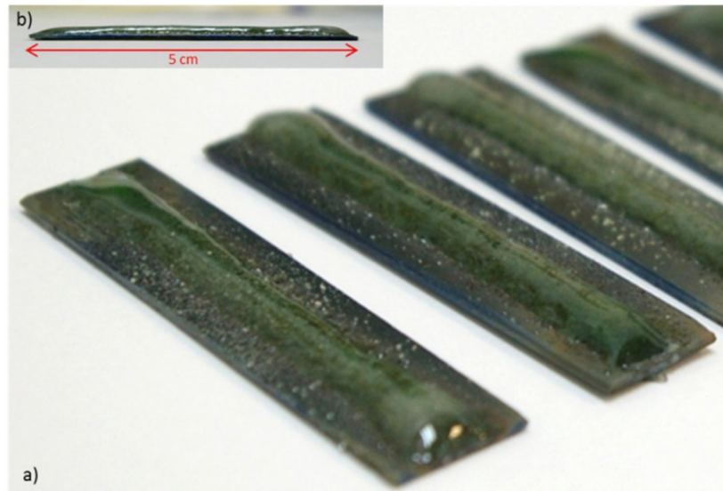
Fig. 2-14. (a) Samples obtained by laser cladding and (b) detail of the thickness [105]
