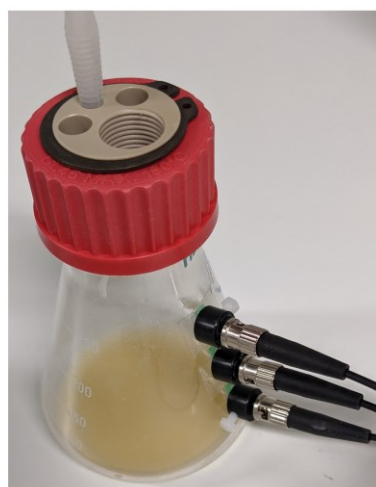
Appendix Figure A20. Erlenmeyer flask for the respiratory activity monitoring system (RAMOS) with three PyroScience optical oxygen sensor spots used to determine oxygen partial pressure p_{O_2} at different heights above a LB-agar cultivation of Escherichia coli BL21.
