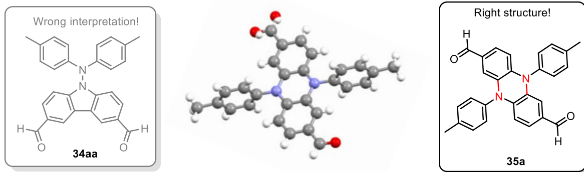
Scheme 8: Comparison of wrong interpretation and the actual structure. [34]
