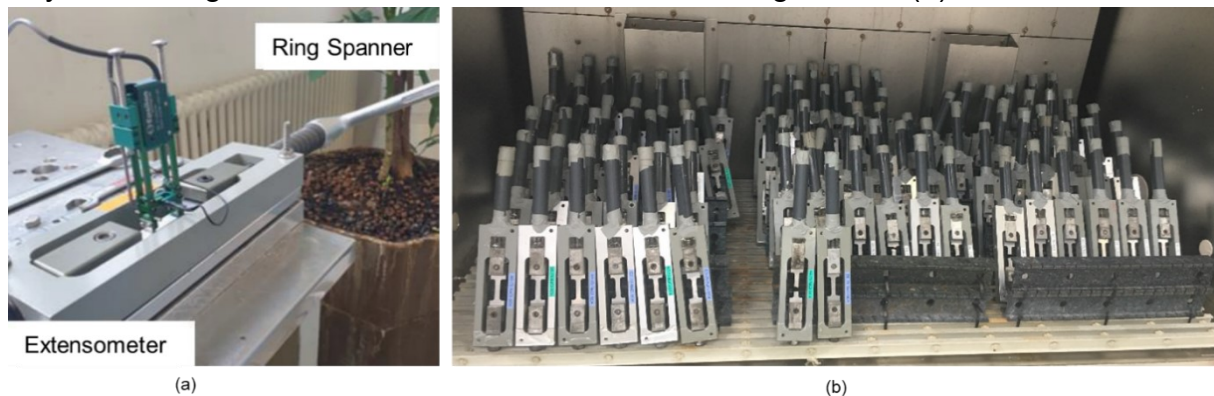
FIGURE 3-10 (A) ILLUSTRATION OF STRESSING OF SPECIMEN USING EXTENSOMETER (B) FINAL EXPOSURE OF SPECIMEN IN THE CORROSION CHAMBER
