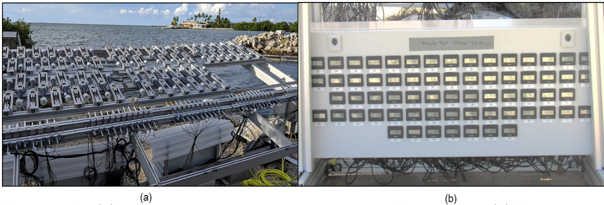
FIGURE 3-16 (A) FINAL SETUP OF TENSILE SPECIMENS AT FLORIDA SITE (B) HOUR METER DISPLAY RECORDING THE TIME-TO-FAILURE OF THE SPECIMENS.
