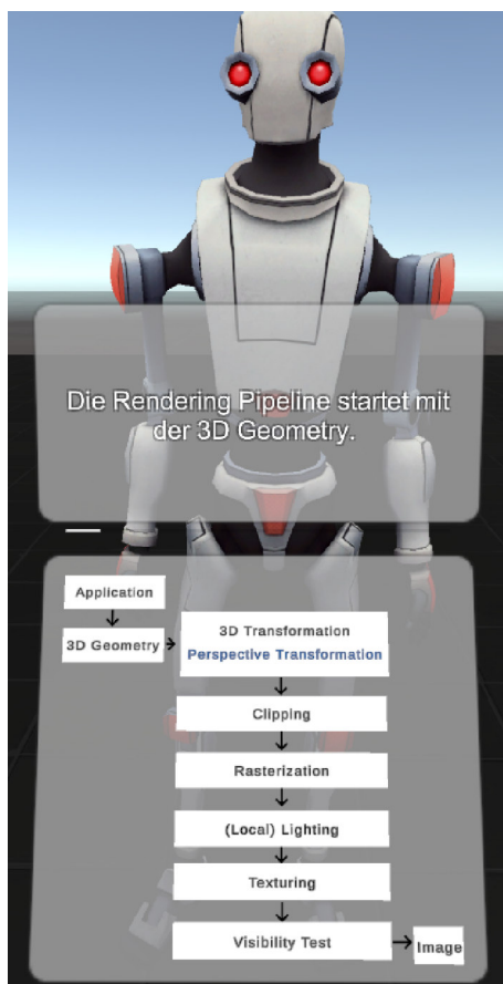
Figure 4.10.: Screenshot from the transformation stage of RePiX VR. Kyle and his text panel are seen in the upper half. The simplified model panel with options to switch between the Rendering Pipeline stages in the bottom half.
