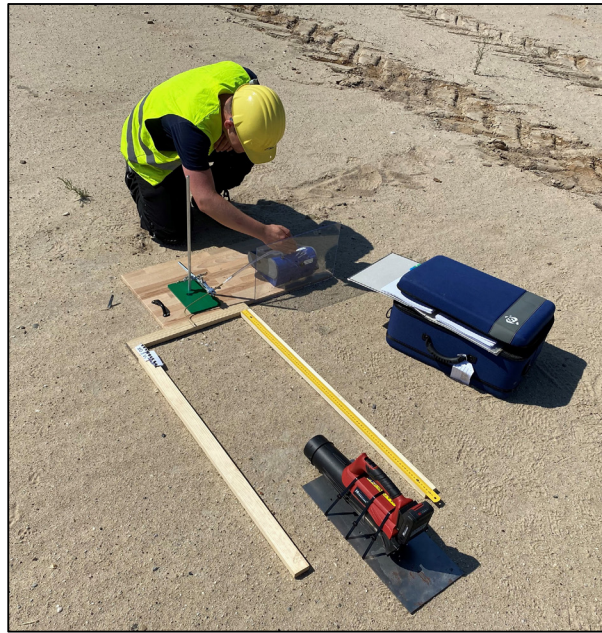
Figure 4.5: Test setup for dust emission measurements.
