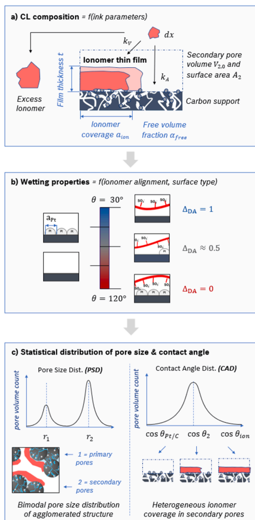
Fig. 1. Schematic of the model workflow: (a) Firstly, CL composition is predicted based on CCL ink parameters. (b) Secondly, wetting properties of the pore walls are estimated accounting for molecular alignment of ionomer side-chains and backbones. (c) Finally, the combined statistical distribution of pore radius and contact angle is calculated, accounting for heterogeneity in ionomer coverage.
