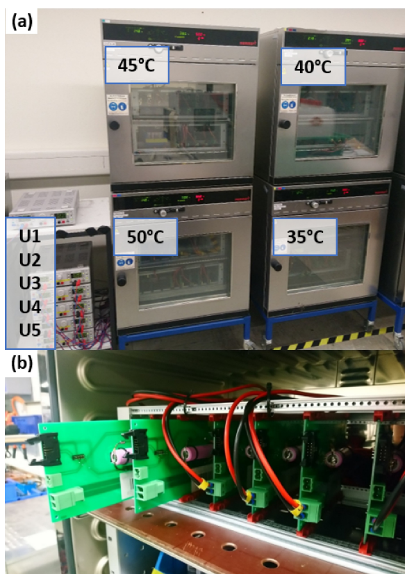
Figure 1. The test setup for storing the cells. 1 (a): 4 ovens at fixed temperatures and the voltage sources on the lower left. Cables from the voltage sources to the cells were run through an inlet on the backside of the ovens. 1 (b): The cells are fixed to a PCB and are stored in racks. The cells were taken out with the PCB boards and connected to the cyclor for the RPT.
