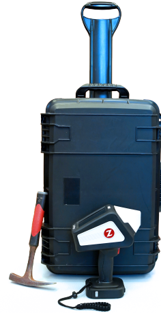
Figure 1.2: Transport case and pLIBS system shown next to a geologist's hammer.
