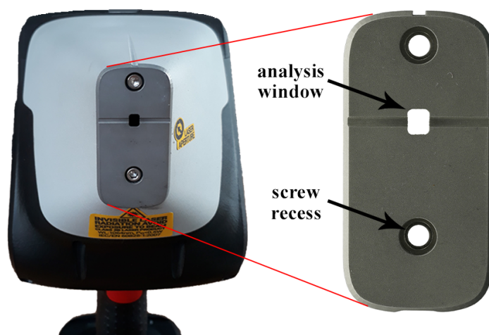
Figure 2.4: The nose of the pLIBS SciAps Z-300. The screw holes and recess next to the analysing window are visible at the front part of the nose.
