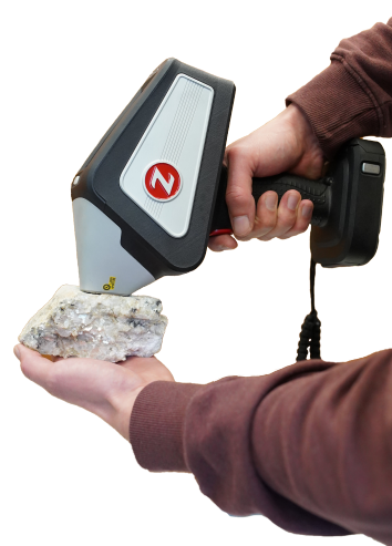
Figure 1.1: pLIBS analysis to determine the lithium content of a pegmatite. Unlike pXRF analysis, the sample can be held in the hand as no ionising radiation is used.
