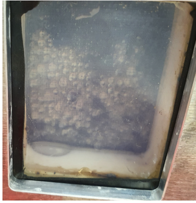
Figure 3.16.: NaOH droplet formation at the back of the sODC facing towards the gas side.
