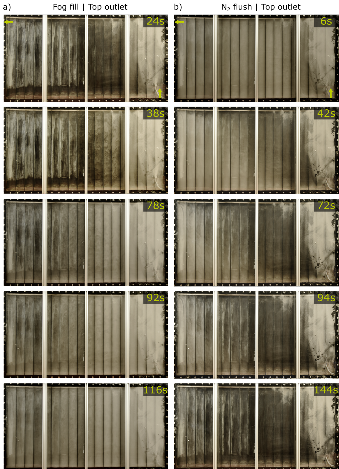
Figure 6.6.: Photos of visualization experiments at different time steps with a) fog and b) nitrogen at the inlet (bottom right) while using the top outlet.
