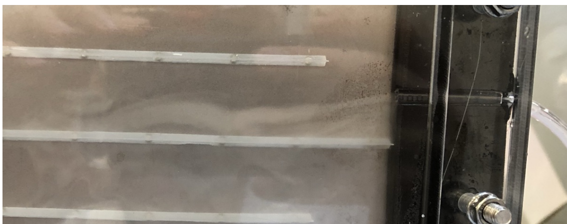
Figure 7.18.: Prototype-cell inlet with fog using the FlowMarker®.
