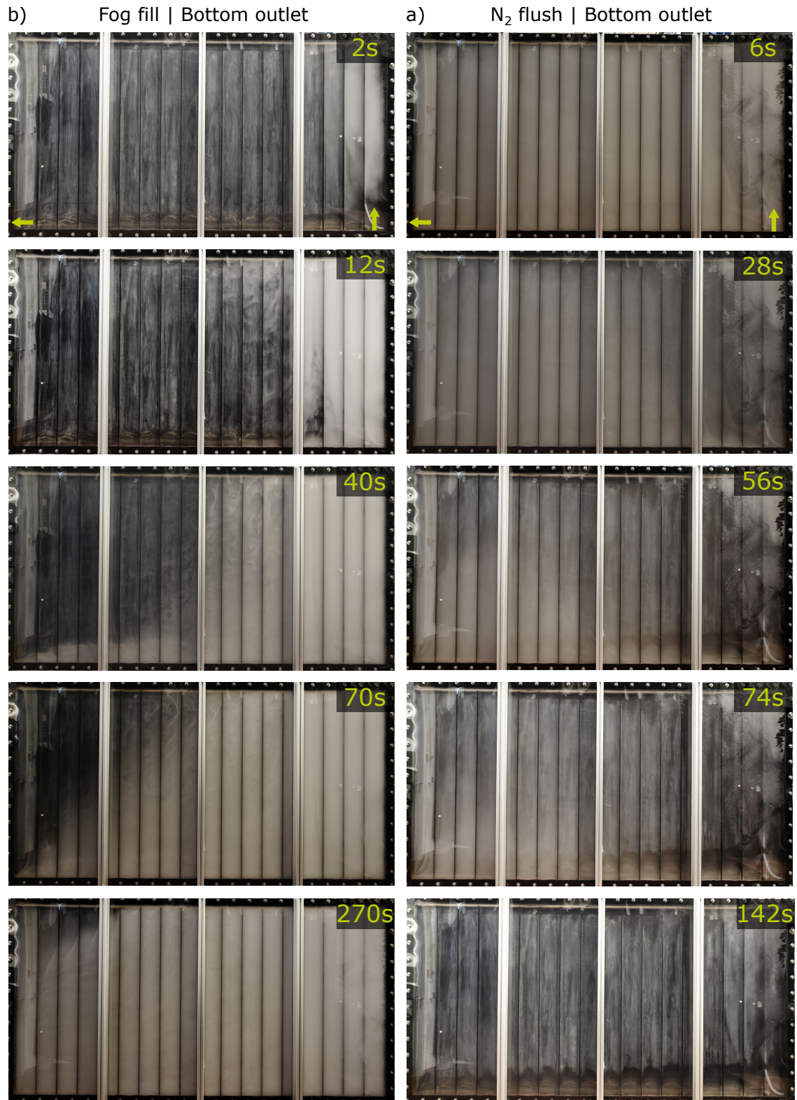
Figure 6.7.: Photos of visualization experiments at different time steps with a) fog and b) nitrogen at the inlet (bottom right) while using the bottom outlet.
