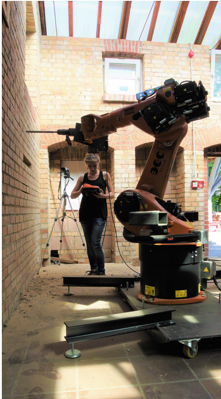
Figure 3.1: An industrial robot KR240 R2700 with a fixed base from KUKA with a customized end effector. The heavyweight (~1100 kg) complicates the on-site application of the robot
