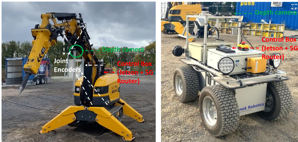
Figure 6.4: Brokk 170 (left) and INNOK 444 (right) with their hardware employed in this project for automated tracking of trajectories and detecting humans
