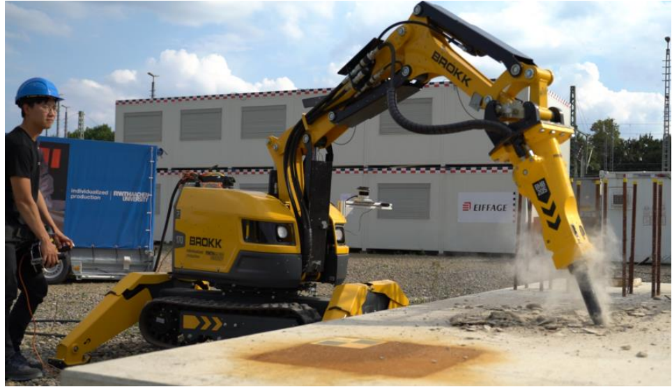
Figure 4.1: Conventional teleoperation, where the human operator directly stands on the deconstruction scene
