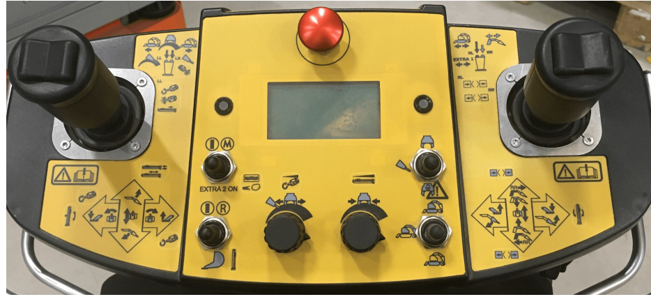
Figure 5.13: Control device for Brokk 170. The left lever controls q_{1,4} and the right lever q_{2,3,5} . When the right button on the right lever is activated, the right lever controls q_2 and otherwise q_{3,5} .
