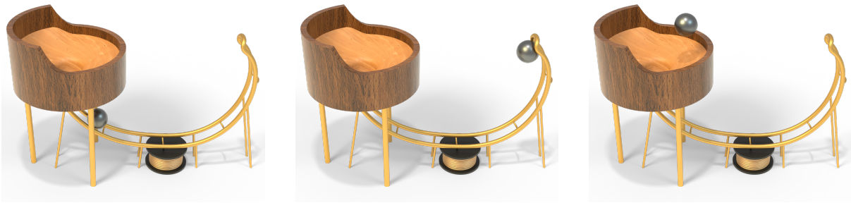
Figure 8: Perpetual Motion Simulator: A magnetizable ball is running indefinitely from the funnel into the tracks and loops back into the funnel. The additional momentum for the ball to loop back into the funnel is provided by turning on and off an electromagnet at the correct time.
