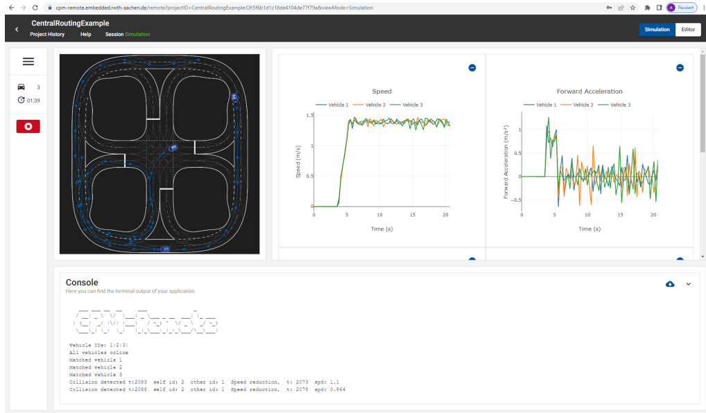
Figure 3.4: Simulation Environment Interface: A visual representation of the CPM Lab’s digital twin, showcasing the real-time simulation of vehicle behavior and scenario visualization.
