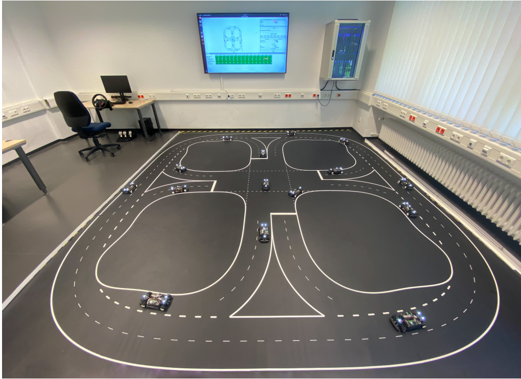
Figure 2.2: A snapshot of the Cyber-Physical Mobility Lab showcasing 15 vehicles on the map. Furthermore, a server rack housing an Intel NUC for each vehicle, a digital twin displayed on the TV screen, and a manual driving steering wheel.
