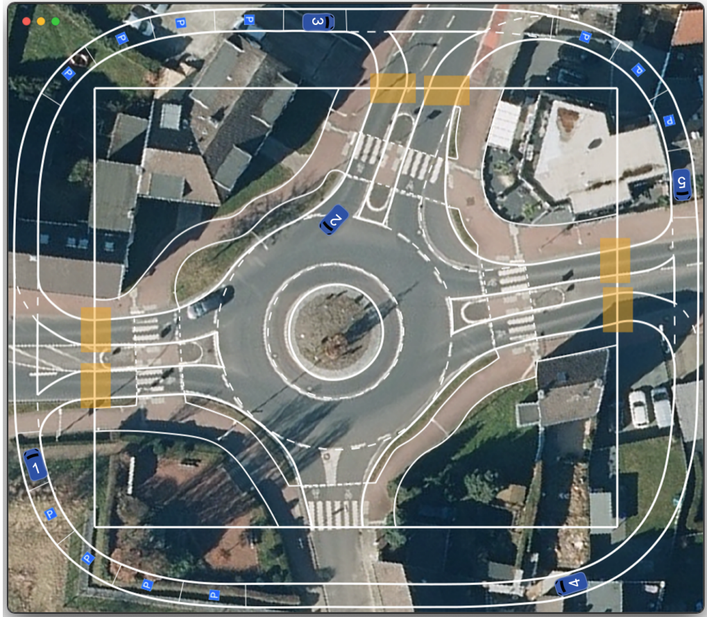
Figure 4.2: Integration of a real-world scenario in CPM Remote, highlighting the boundary (white rectangle) and transition zones (yellow areas) between system-managed and user-managed planning areas.
