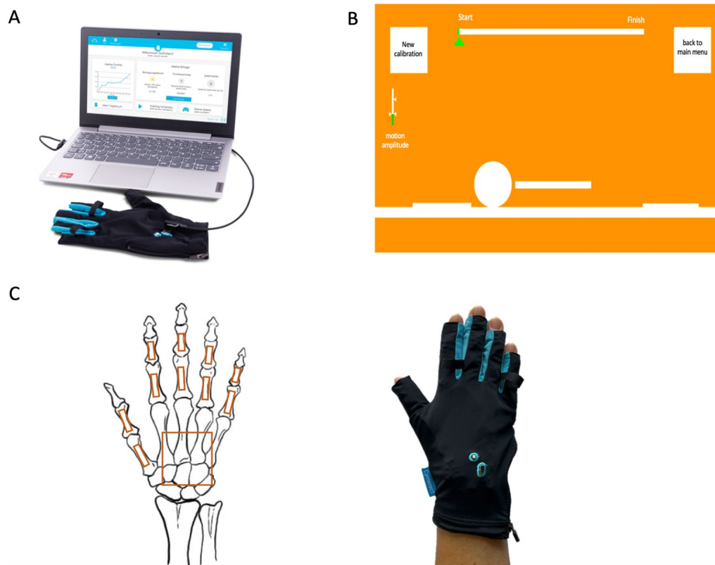
Fig. 1 Overview on the technical and functional background of the glove. The data glove was connected to a computer/laptop running the corresponding software (A). Patients had to complete a course and its alternating obstacles by adjusting the size of a sphere, that was controlled by finger movements. To the left of the screen, a green bar indicated the current motion amplitude based on calibration. At the top, a progress bar specified the position within the course. The button in the upper right corner allowed for cancellation of the game and for returning to the main menu (B). Sensors for data acquisition were located over the dorsal sides of the proximal, resp., the middle phalanges of the long fingers. For the thumb, they were fixed at the first metacarpal bone and the proximal phalanx. The larger main board sensor was placed on the dorsum of the hand in the region of the metacarpus and the carpus and served as the central reference point for the proximal phalanges of the long fingers, as well as for the first metacarpal bone. Corresponding to the anatomical bone structures, on the right, the glove is shown as being worn (C)
