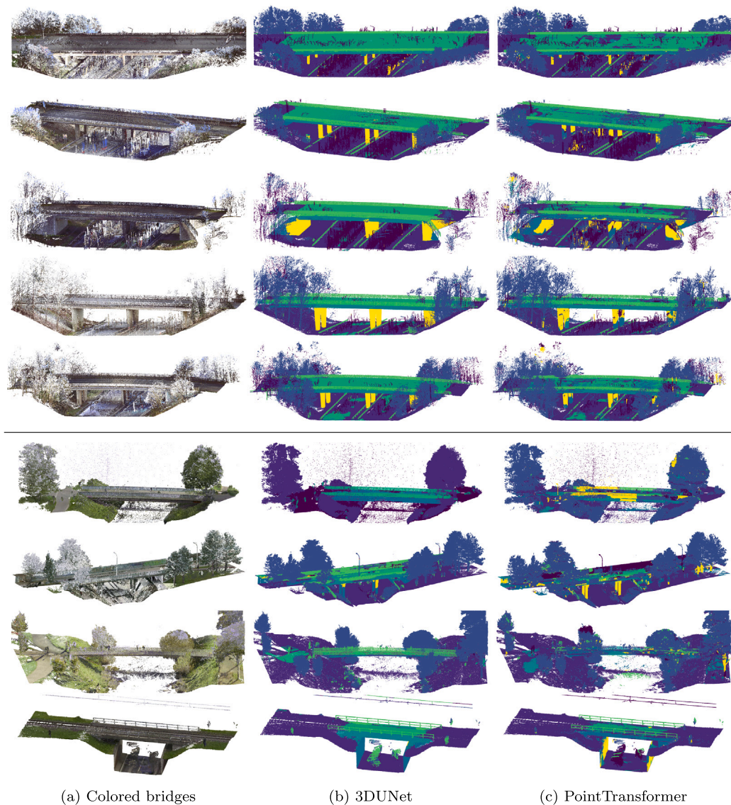
Fig. 10. Prediction results using the SSDA approaches. The Section 1 presents the outcomes of the data provided by [25]. The Section 2 presents the outcomes of the data recorded on bridges in Freiburg, Germany using a different sensor. Color code is defined in Table 2.
