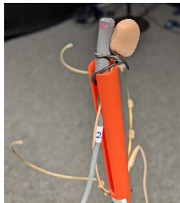
Figure 6.3: Set up of the latency measurement. The microphone used for the listening test was taped to a reference microphone.
