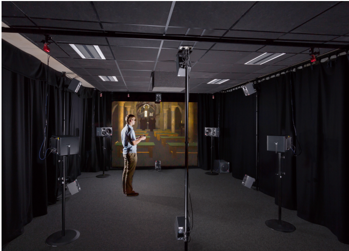
Figure 3.1: Picture of the VR-Lab and equipment setup. Twelve loudspeakers in three horizontal rings with different elevation can be seen. Visible acoustic measures are the acoustic ceiling as well as the curtains, which can also cover the screen. The box in the ceiling contains two projectors for visual stereoscopic presentation via polarization. The red cameras in the ceiling are part of the tracking system. The user is equipped with tracked glasses and a (tracked) game pad for interaction. The forward direction is towards the screen. Copyright at Institute for Hearing Technology and Acoustics, RWTH Aachen University, Germany
