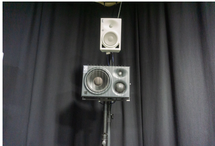
Figure 4.3: Reference position two and the front right loudspeaker (horizontal plane) of the loudspeaker array. Both position share the same azimuth angle, but differ eleven degrees in elevation.
