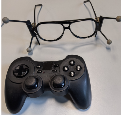
Figure 3.2: Picture of the tracking glasses used in the VR-Lab, the polarization lenses are removed. The tracked point is the geometric center of the triangle spanned by the four white tracking markers. This point was shifted in post-processing to match the center point of the aural axis. The game pad was used as an input device to pan virtual sources.
