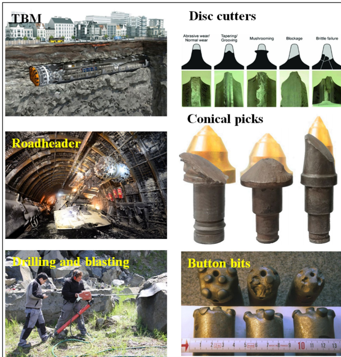
Fig. 1 Wear of typical mechanical tools (e.g., TBM discs, roadheader picks and drill bits) during hard rock excavations. (Thuro 1996; Thuro 2002; Ellecosta et al. 2018; Janc et al. 2020; Zhang et al. 2022b; Bołoz and Biały 2023, modified)
