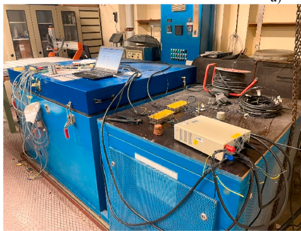
Fig. 11. Test setup for the freeze-thaw exposure: a) Technical drawing – circuit; b) Overview of climatic chamber; c) Overview of tensile specimen in climatic chamber.
