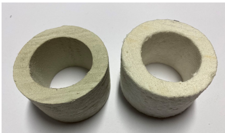
Figure A.1: Original shape of the filter candles used in the exposure experiments. Ca-Mg silicate fiber filter candle (l.) and Al-oxide silicate fiber filter candle (r.).
