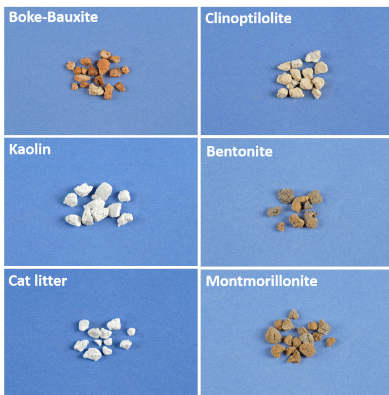
Figure 3.7: Visual appearance of alkali sorbents before sorption experiment (grain size: 1.6–4 mm).
