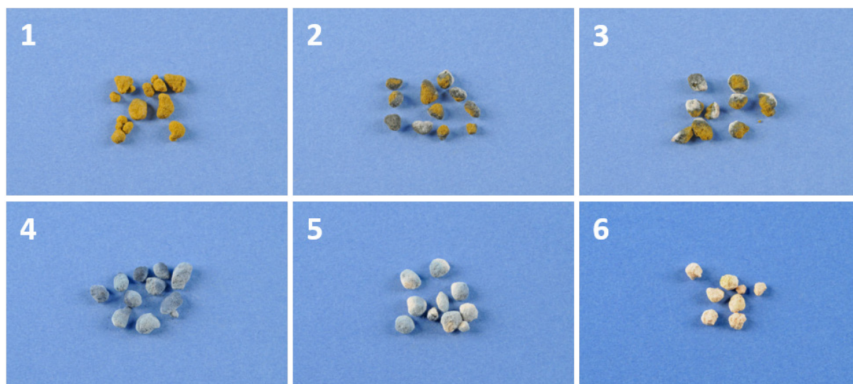
Figure 3.14: Cerium oxide samples after exposure in a 10 %-H 2 -Ar atmosphere at 1500 °C for 72 h. Only cerium oxide samples corresponding to picture 1 were used.
