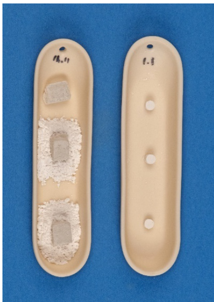
Figure 3.17: Filter candle pieces embedded in sorption material (l.) and filter candle-sorbents pellets (r.) before exposure.
