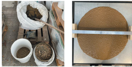
Figure 2. Sieving and preliminary testing of the poured earth mixtures.
