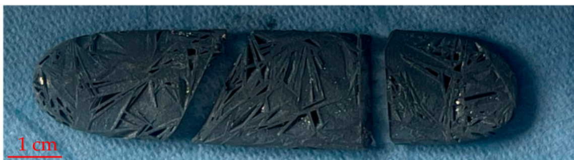
Figure 11. Reaction products after reducing at 800 °C for 2 h.
