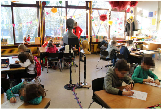
Figure 2.2: Example of the centered positioning of the measurement transducers during an in-situ measurement in a classroom (Loh et al., 2022b).
