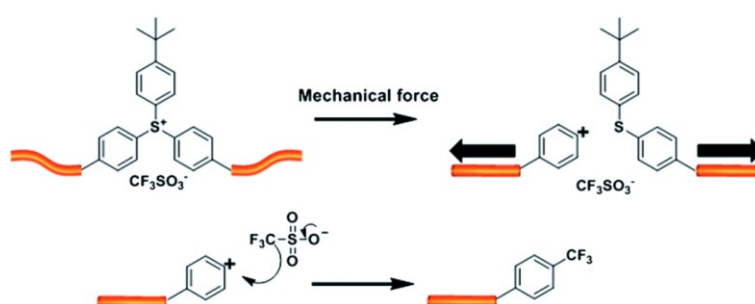
Figure 24. Ultrasound-induced heterolytic scission of the C–S bond in the triarylsulfonium salt (TAS) moiety. Adapted from ref. 66. Copyright © 2014 The Royal Society of Chemistry.
