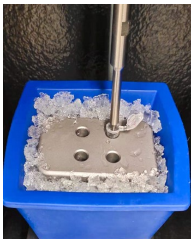
Figure S14. Unfocused US setup ( f = 20 kHz, with ice bath). Temperature record: 0.3 °C (before sonication), 2.1 °C (after 10 min sonication).
