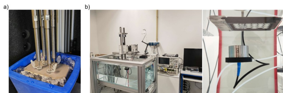
Figure S5. Sonication systems. a) 4-probes 20 kHz sonicator. b) HIFU sonication system (left), transducer and 24 wellplate (right).
