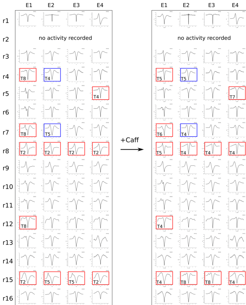
Figure 5.23 – IRB sample at DIV 26 spike shape change upon caffeine addition. A total of 14 electrodes detected a different STA upon addition of 8mM caffeine. The change is complete in only two rows: r8 and r15. In blue rectangles are shapes that did not change significantly, i.e. remained within the same group of triphasic shapes. The red rectangles are shapes that underwent a visible change in shape by also belonging to different groups of spike signals.
