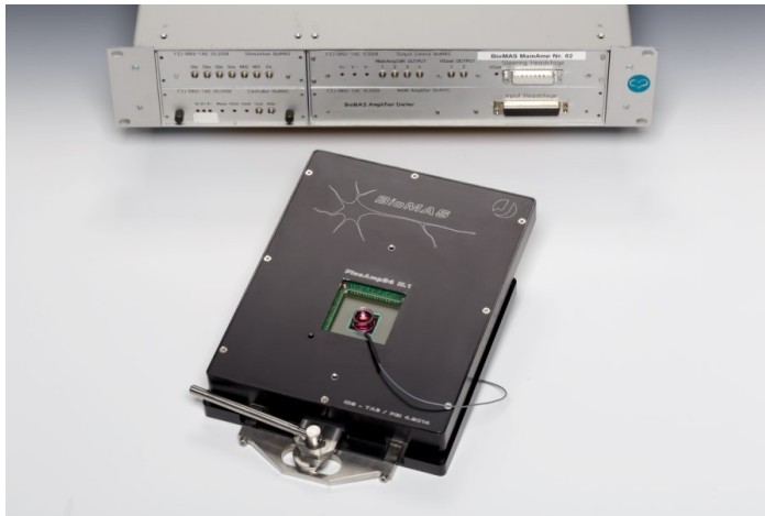
Figure 2.8 – BioMAS recording setup: the main amplifier, headstage, and MEA chip with a growing cell culture. This custom amplification system was designed and developed at the institute as a part of a doctoral thesis (Eick, 2009).
