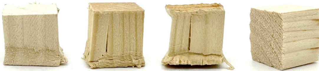
Figure 2. Typical failure mode occurred during compression tests. Left: crushing failure of raw spruce specimen (CS_C1_P1_126); Mid-left: crushing and splitting failure of Ga_M (CS_C1_P2_54); Mid-right: end rolling, crushing and splitting failure of Ga_M_f (CS_C1_P2_41); Right: compaction and wrinkling of raw specimen (CS_C1_P1_111).
