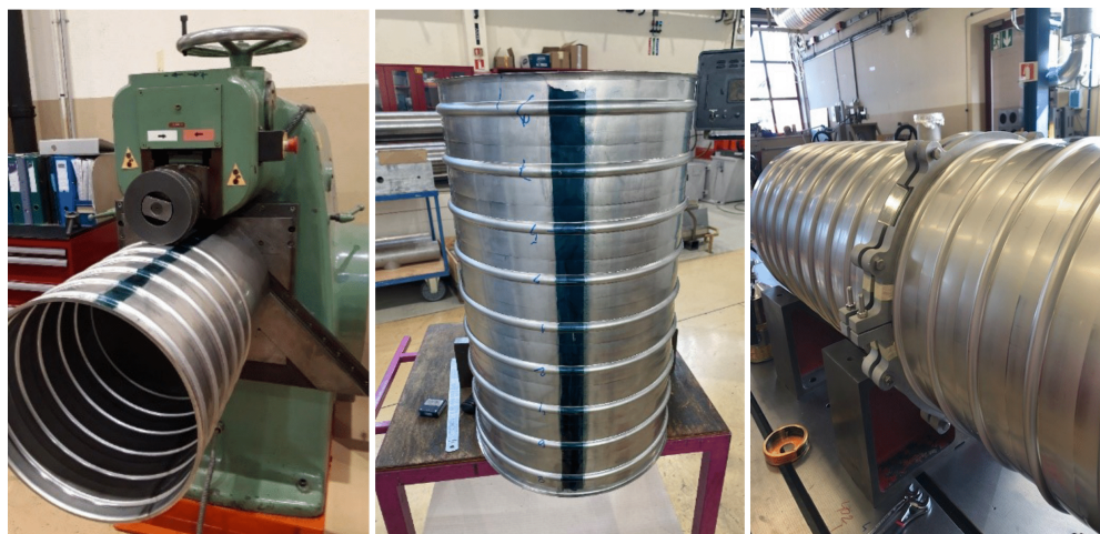
Figure 5.1: Pictures of the corrugations steps for one AISI 304L section and final alignment for the butt welding for the final chamber production. Courtesy of Gilles Favre (CERN).
