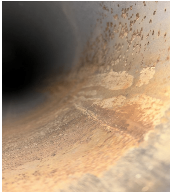
Figure 6.32: Internal surface aspect after the two heating cycles. Compared to Fig. 6.29, the oxide patches darkened in colour.
