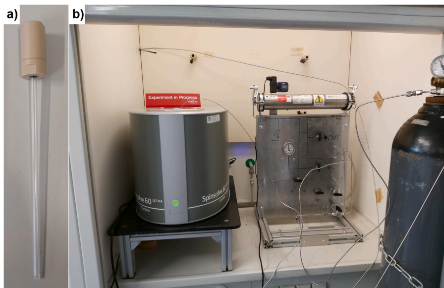
Fig. 1. Photograph of a) the HP sapphire tube proposed in Ref. [47] and b) the HP-setup and the employed benchtop NMR device introduced in Ref. [46], placed together inside a fume-hood.
