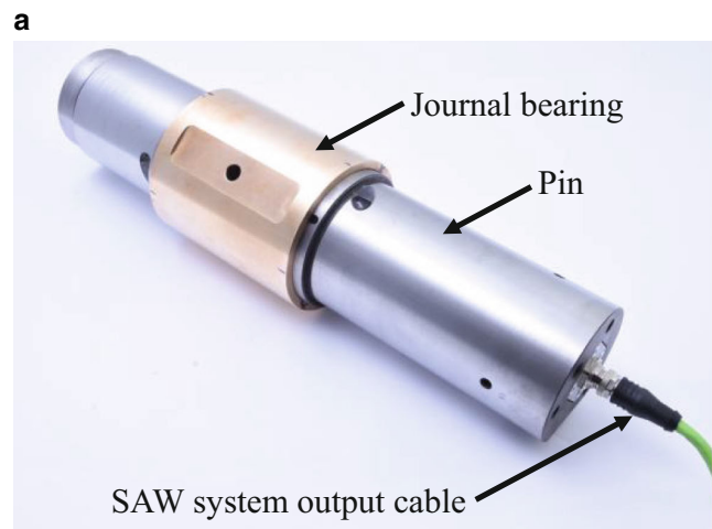
Fig. 5 SAW sensor setup on the planetary journal bearing test rig (PJB) relative to the pressure distribution
