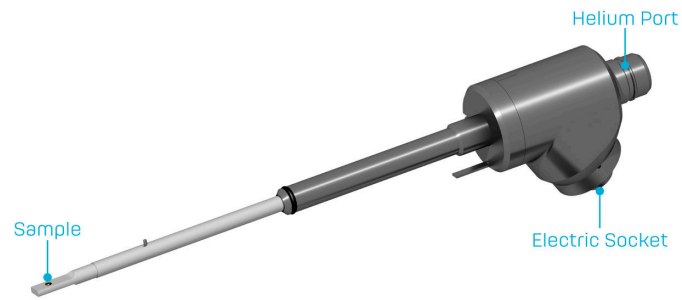
Fig. 2.13: Sample holder of a TEM is utilized to put and hold the sample during the data acquisition or measurement. The liquid helium flows to the sample holder to reach a lower temperature (down to 4-5 Kelvin). The image is adapted from [90].
