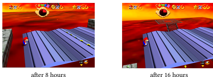
Figure 5.6: Upwards moving platform in Super Mario 64 due to rounding errors caused by Round to Zero (RTZ). Footage from [180].
