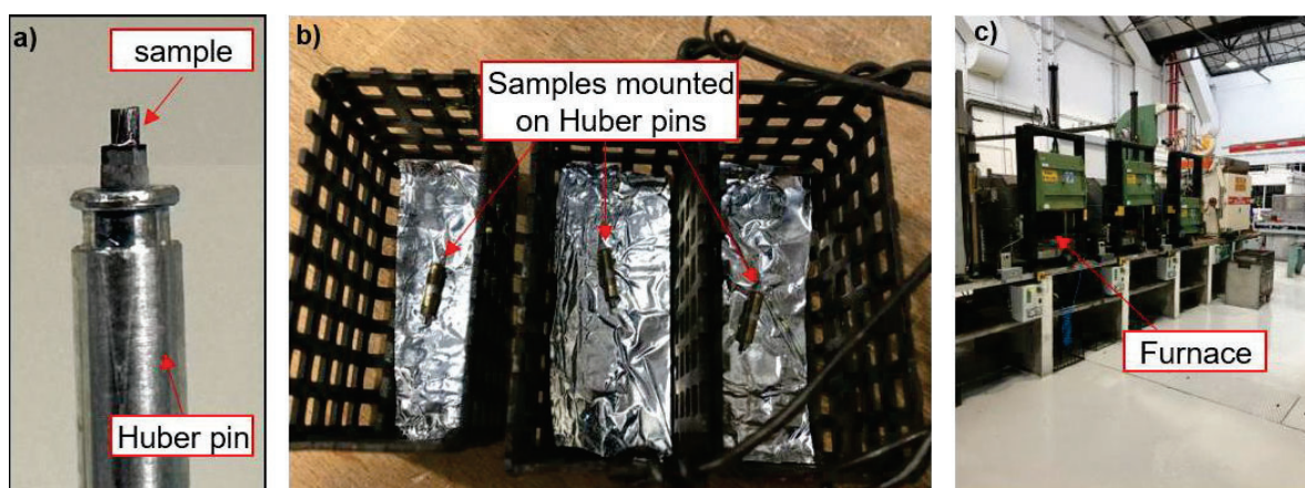
Fig. 5.4 Samples subjected to heat treatment at Constellium at 400^{\circ}\text{C} for 4 hours. (a) Sample mounted on the Huber pin. (b) Individual samples placed in designated crucibles. (c) Industrial furnace utilized at Constellium for the heat treatment process.
