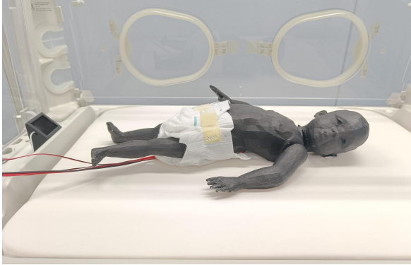
Abbildung 6.2: Test bench with neonatal phantom and reference body inside the incubator.
