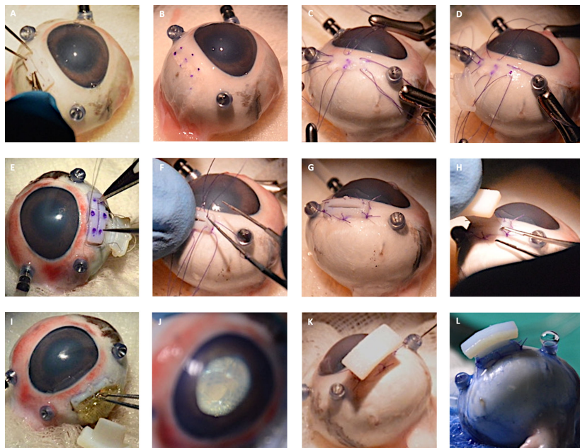
Figure 3. Porcine eye. Ophthalmological vitrectomy setup consisting of three 23G trocars (EVA AVETA23G Cannula set with high flow infusion line, Article No: 1272.ED23, D.O.R.C. Dutch Ophthalmic Research Center (International) B.V., Zuidland, The Netherlands), running infusion, marking of 6 suture points with surgical marker using 3D-PLAPS pre-implantation template (A, marked in B), suturing process with 6-0 Vicryl surgical suture (ETHICON; Johnson & Johnson, New Brunswick, NJ, USA) and stabilized by 2 Dieffenbach serrifine forceps (Geuder AG, Heidelberg, Germany) (C), attachment of 3D-PLAPS device onto 3 bottom sutures (D), use of pre-implantation template for marking of incision points, scalpel (size 11) incision (Feather disposable scalpel, Feather Safety Razor Co., LTD, Osaka, Japan, Socorex Isba SA, Ecublens/Lausanne, Switzerland) (E), scleral fixation of 3D-PLAPS with 6-0 Vicryl surgical sutures (F), result of attachment (G), adapting the closing plug to the device (H), implantation of VLARS epiretinal stimulator dummy through 3D-PLAPS and correct positioning inside eye cavity epiretinally (I, J), trypan blue tests for sealing and leakage (Vioron Vial 0.5 mL, G-81001, 1000188, Fluoron GmbH, Ulm, Germany), semi-quantitative flow analysis inside eye (K, L) (showing the closing plug on 3D-PLAPS with leakage of the infusion trough 23G trocar system).
