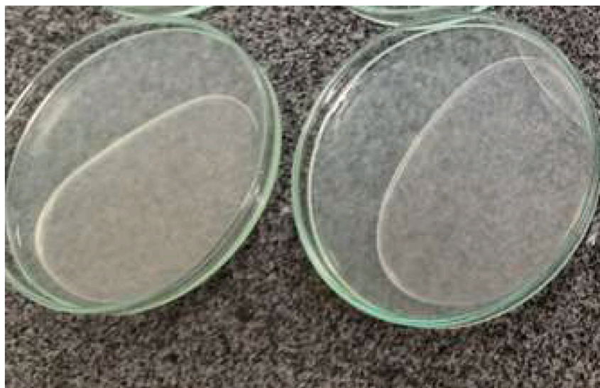
Fig. 1. Vinyl ester resin sample (R3) with air pockets between the layers when produced in petri dishes.
