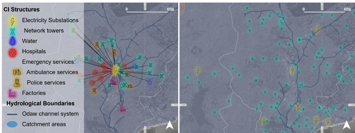
Figure 2-10: Critical infrastructure network elements involved in flood mitigation measures in and around the Odaw river system. (Left) In the centre, an electricity substation is highlighted which is connected to 43 sink elements. (Right) Mobile network towers and electricity substations.
