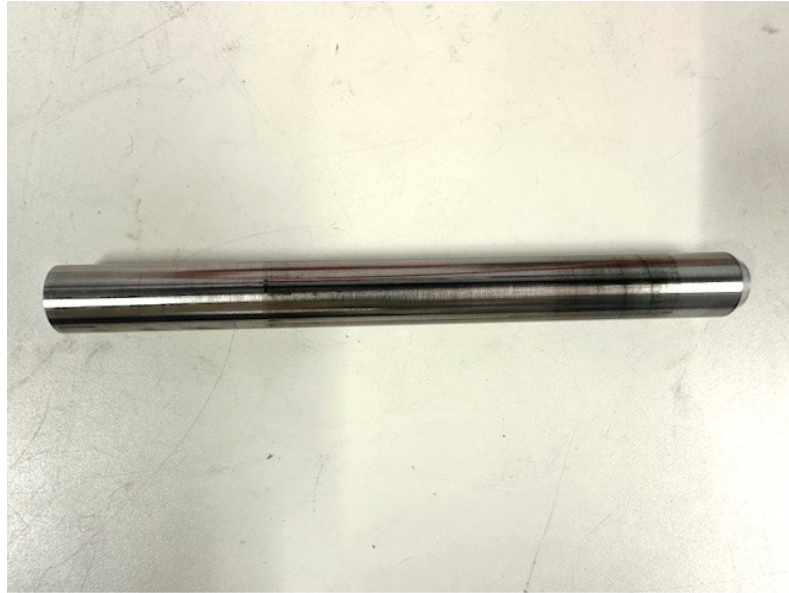
Figure B.1: Image of a rough rod used for testing at ambient temperature after 4 days of use. Black PTFE film is observable on the surface.
