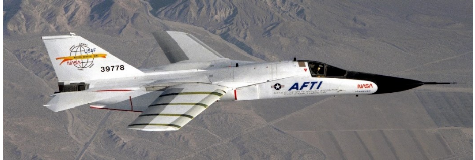
Figure 2: General Dynamics F-111 Aardvark with mission adaptive wing [22].
