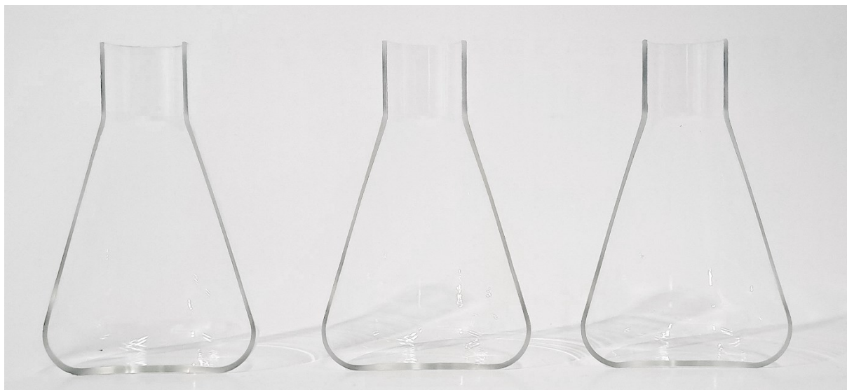
Appendix 2: Shake flasks milled to half their maximal outer diameter to evaluate the exact geometry of the flasks.
