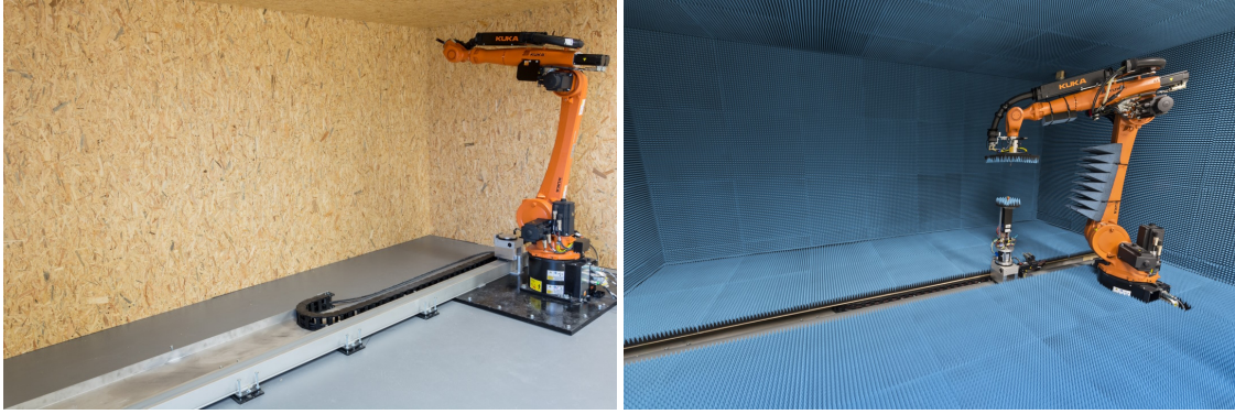
(a) Actuators directly after integration on common ground plate and renewed floor. (b) Operational measurement system including setups for AUT and probe.
