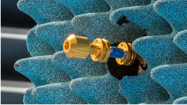
Figure C.3: Picture of the SFH antenna mounted in the CATR of the IHF.
