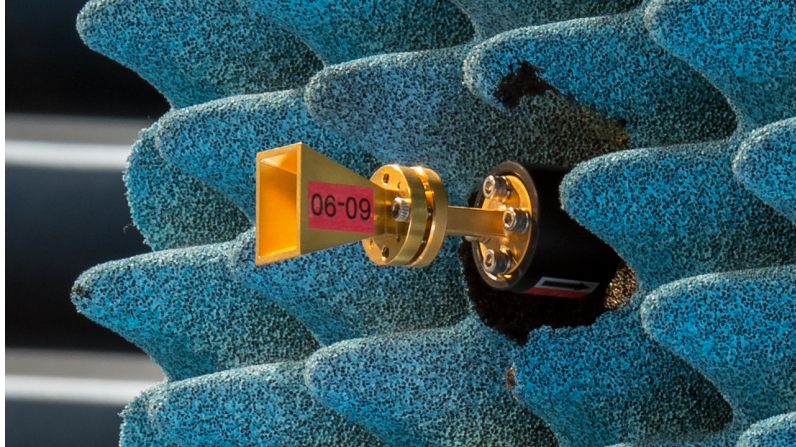
Figure C.1: Picture of the AUT used during the reference measurements performed in the CATR of the IHF.
